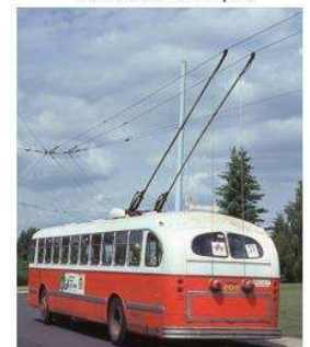
Trolley poles connected to retrievers with ropes
