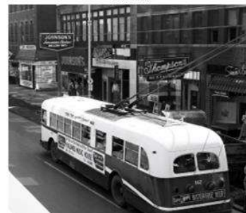
View of trolley poles mounted on roof
